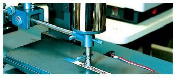
Abrasion resistant: after a 1kg sanding device was passed over the laminated labels 50 times, the text was unaffected.
